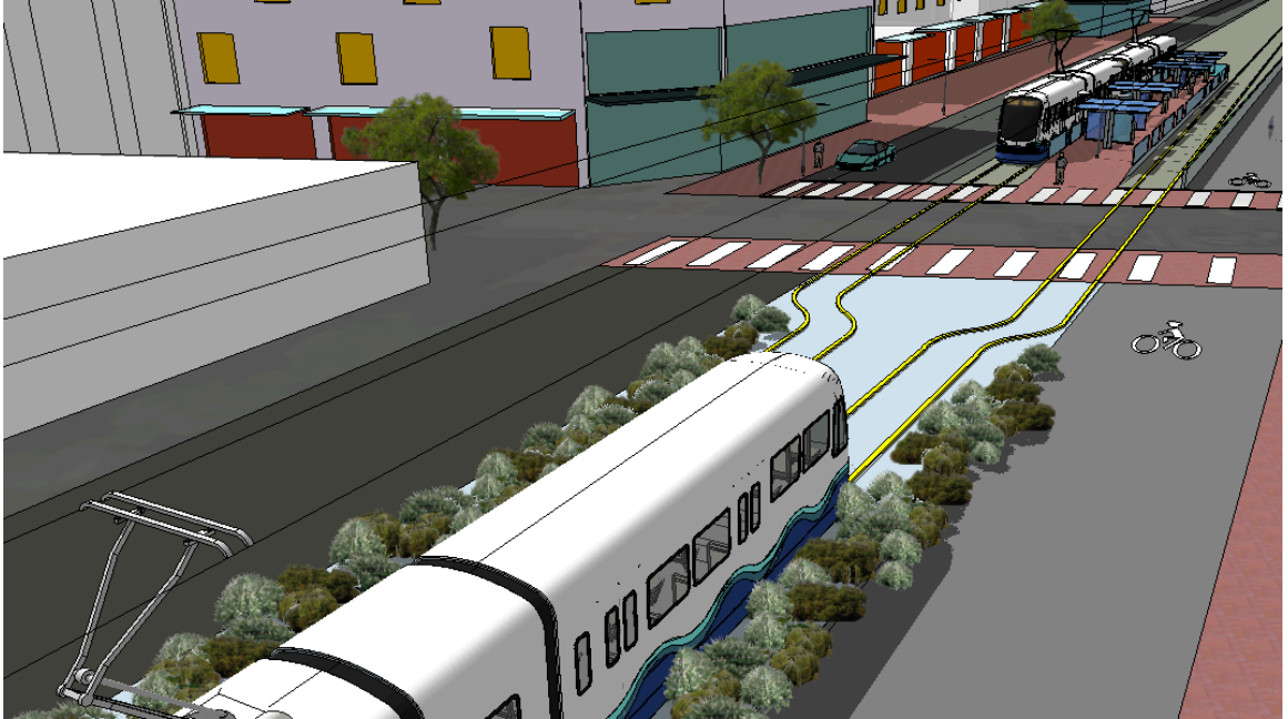
FIGURE 11. Given the limited space between car traffic on NE 76 th Street and the Redmond Connector Bike Path, the light rail tracks will split immediately before and after stopping at the station to allow for a larger, shared platform in the center of the tracks. The tracks will meet up on either side to allow room for a vegetated buffer between car and bike traffic along the rest of the line.
