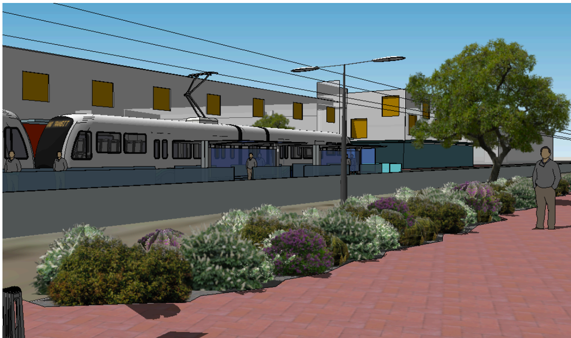
FIGURE 13. A number of bioswales will be put along the plaza to help retain and filter stormwater runoff, and the plaza itself will be constructed out of interlocking permeable pavers.
